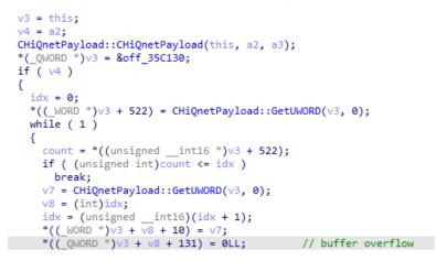
Figure 5.12: Vulnerability in CHiQnetPayloadMultiSvGet::CHiQnetPayloadMultiSvGet()
