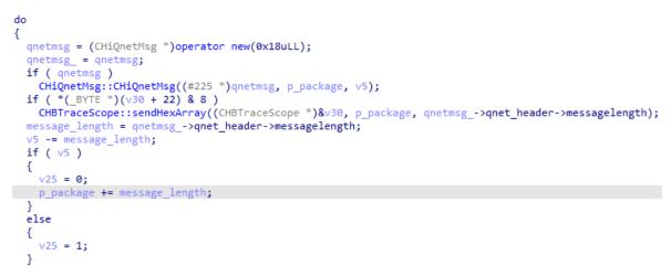
Figure 5.9: Vulnerability code snippet of function ComPort::processTcpMessage
