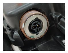
Figure 9.5: Gas generator pins
