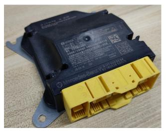
Figure 9.3: Airbag control module
