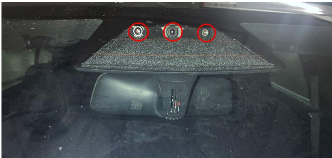
Fig 6. “main”, “narrow” and “fisheye” camera on the vehicle.
