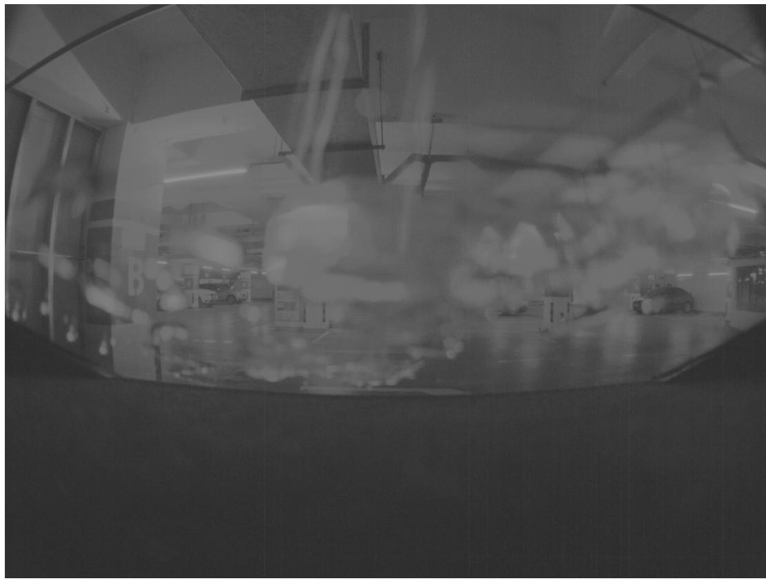
Fig 14. Picture of the water on the windshield captured by the fisheye camera.
