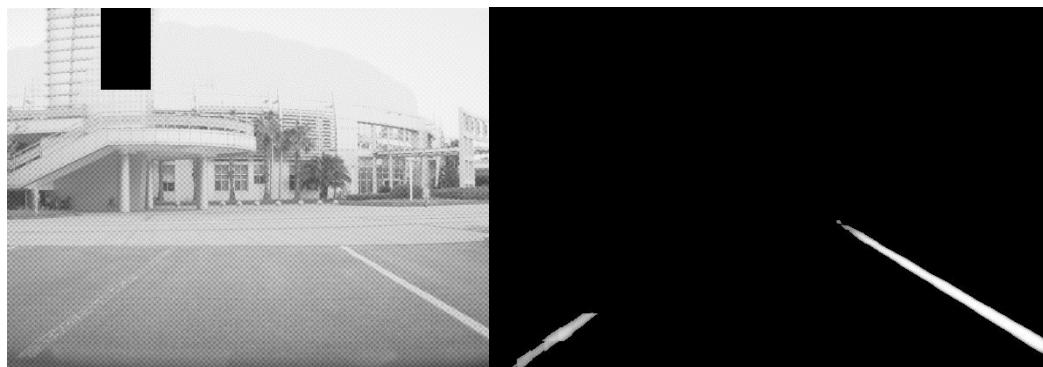
Fig 29. Left picture shows we add some noise on the left lane line in digital level, and right picture shows the result of APE's lane recognition function. (We redact top left of our image for privacy reasons, but it won't affect the final result.)
