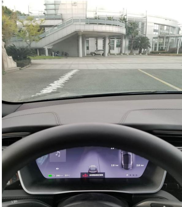
Fig 32. adding some patches around lane line in physical world, and there is only right lane in the CID (central information display)
